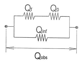
Recalling that conductances add in parallel while resistance add in series, we can immediately write down an expression for  $Q_{obs}$  as a result of the resistive model diagrammed above:
