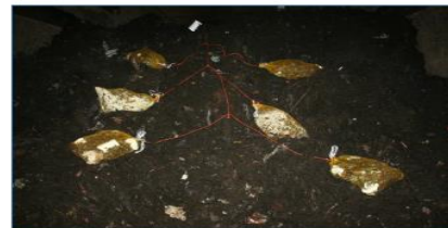
Figure 11 Position of the mesh bags in the composting tunnel (Trial 5).
