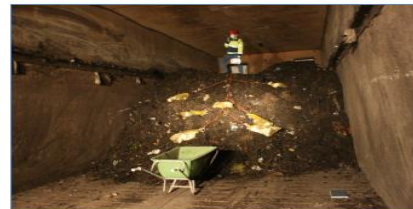
Figure 10 Placing the mesh bags in the composting tunnel (Trial 1).
